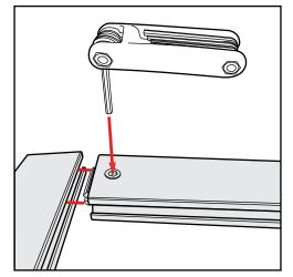
Extrusion & Lock Connection
